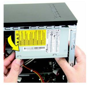
To install the power supply, reverse the removal procedure. Note that there is a latch, a guide, and a ledge on the computer that help secure the power supply.
